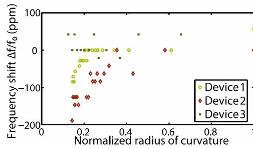
**Figure 6.** Relative frequency shift versus normalized radius of curvature versus temperature from wireless reading.
