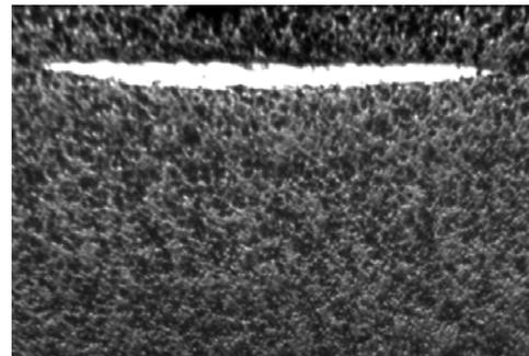
**Figure 4.** Light microscope cross-section view of one turn (bright) of the planar loop with the embedding layer on top.
