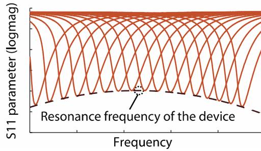
**Figure 2.** Frequency sweep of the loop antenna when placed 5 cm above a device. The resonance frequency of the latter is found at the maximum of the fitted line.
