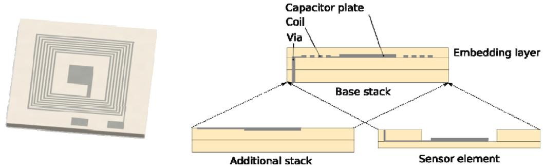
**Figure 1.** Tilted top-view of the top-layer of the device (left), and a cross-section schematic divided into: base stack, the additional stack and the pressure sensor element (right).
