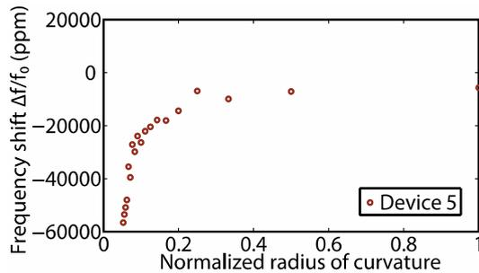
**Figure 7.** Relative frequency shift versus normalized radius of curvature versus temperature from wired reading.
