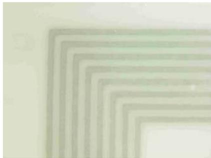
**Figure 3.** Stereo microscope close-up image of the planar loop through the embedding layer.
