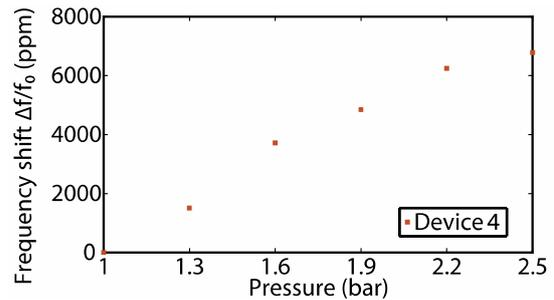
**Figure 8.** Relative frequency shift versus pressure from atmospheric pressure to 2.5 bars.
